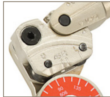
Roller dies reduce force and tube flattening.
